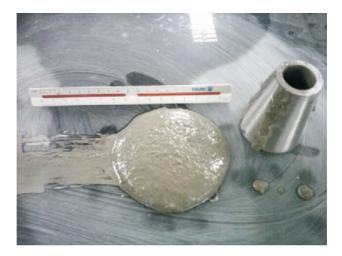
Figure 3 - Mini-slump test (Laister, 2012).
