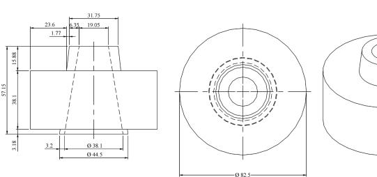
Figure 2 - Project design of mini-slump apparatus (units in mm) (Based on Kantro, 1980).
