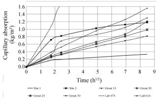
**Figure 5** - Capillary absorption of the mortars studied (Laister, 2012).
