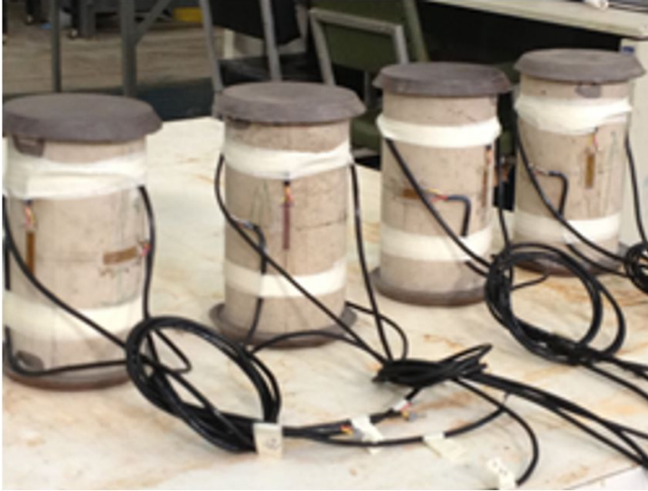
Figure 9: Technological control of the block and pile concrete.
