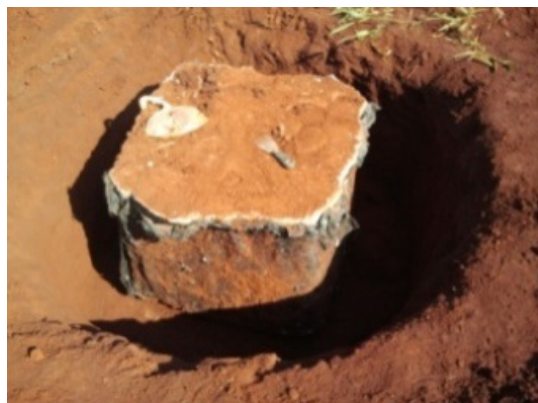
Figure 10 DPR_{(EXP)} system excavated laterally.
