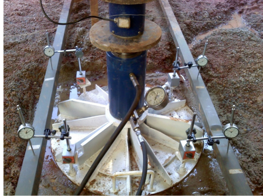
Figure 5. Assembled load test.
