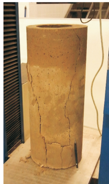
Figure 22 - Sample after failure stage (laboratory test).
