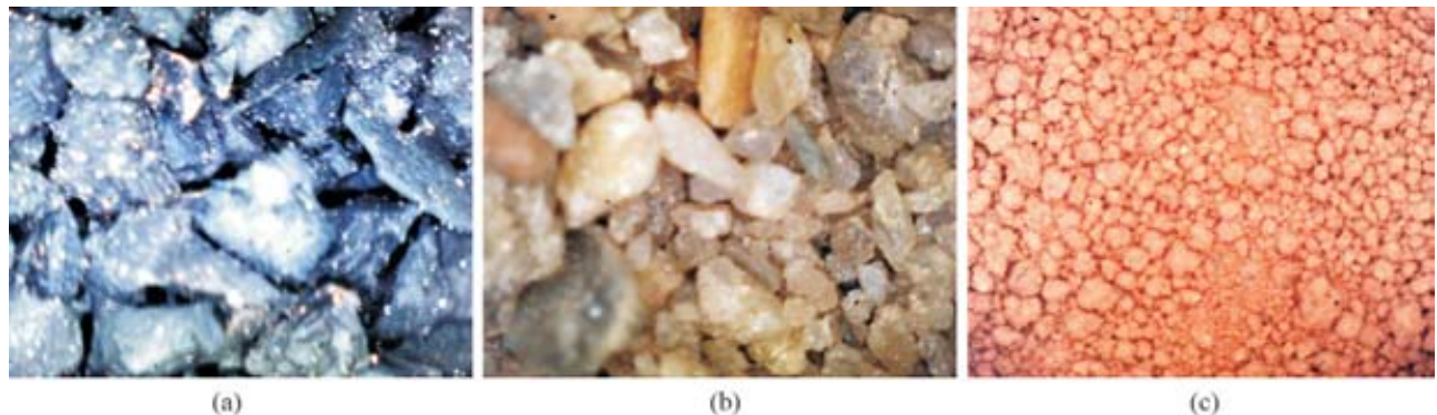
Figure 1 - Materials mixed with the bentonite to produce the alternative GCLs: (a) Tire grains (TG); (b) Sand (SND) and (c) Clay (CLY) - 50x enlargement.
