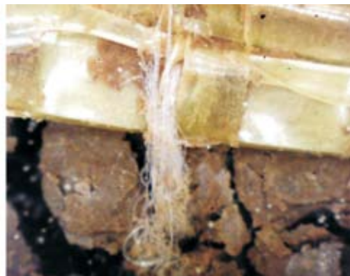
Figure 18 - Stitches of GCLs A and B after hydration: (a) GCL A stitch after hydration; (b) Failed stitch in GCL B after hydration.
