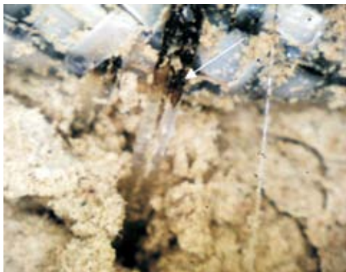
Figure 18 - Stitches of GCLs A and B after hydration: (a) GCL A stitch after hydration; (b) Failed stitch in GCL B after hydration.
