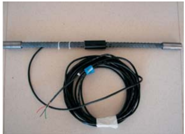
b) Instrumented steel bar
