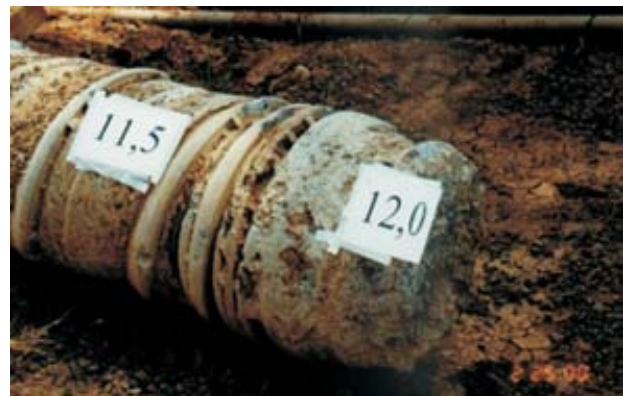
Figure 31 - Omega 2 pile tip characteristic.
