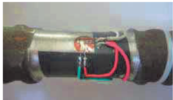
Fig 12. Wheatstone bridge connection
