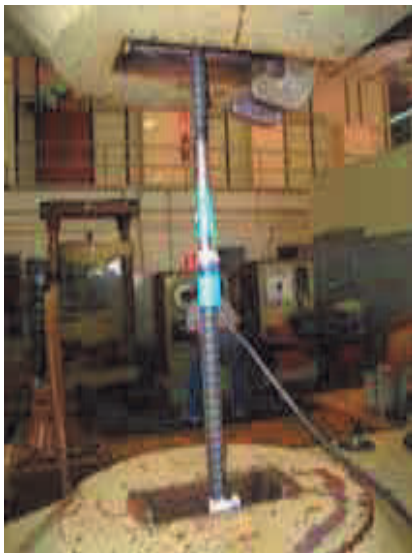
Fig 13. Checking the bar on a tensile testing press
